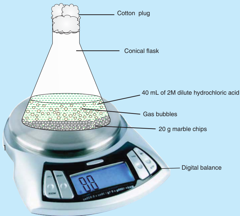
Figure 4.1 Laboratory set up for the measurement of rate of reaction.
